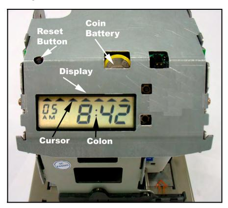
Figure 2-18. Auto-Sync Time Clock Front Panel.
